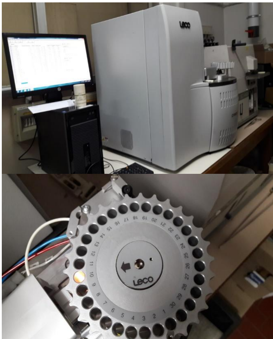
Figure 13 – Elemental analyzer CHN 628 manufactured by LECO in operation (instrument is used at the Institute for Research on Combustion in Napoli, Italy)
