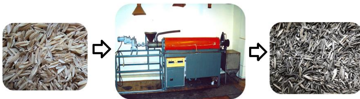
Figure 8 – Rice husk carbonization in auger furnace
